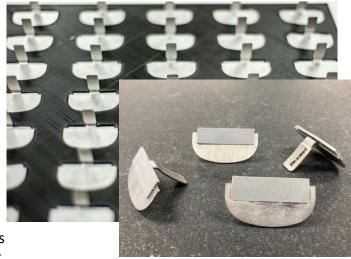
BACK: 3D printed precision assembly fixture used to position the rubber seal into place before adhesion IAW the drawing specifications. FRONT: Assembled seals demonstrating the rubber adhered into position IAW resistant stainless steel. the drawing. Images provided by Parts Life, 2021.
